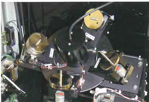
* Automatic probe exchanger among 4-kinds of probe head
