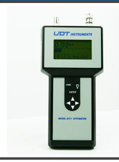
The model S471 High Performance Handheld Optical Meter is ideal for photometric, radiometric, laser power, and fiber optic measurements. Designed to be used in a laboratory setting or field environment, the microprocessor controlled architecture features direct analog display, serial RS-232 output and analog voltage output.
