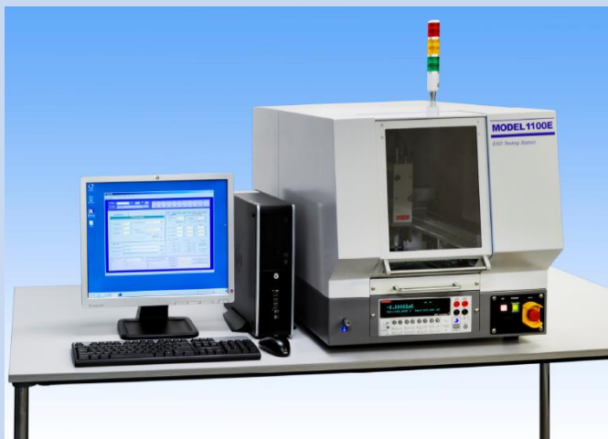
Model 1100E (High Pin count ESD Tester without supporting Pin Combination Test)
