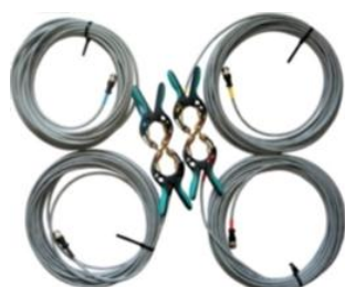
H winding test cable set
