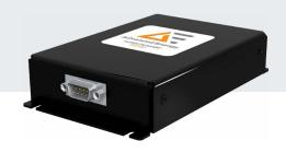
The HiTek Power® PSM10 series is a range of versatile high voltage component power supply modules equally suited to both laboratory and development work, as well as for specification in OEM equipment. Powered from 24 VDC, these units allow full range control and monitoring of voltage and current via 0 to 10 V analog signals and inhibit signal input. Positive or negative polarity models up to 15 kV are available with customer-defined derivatives upon request.
