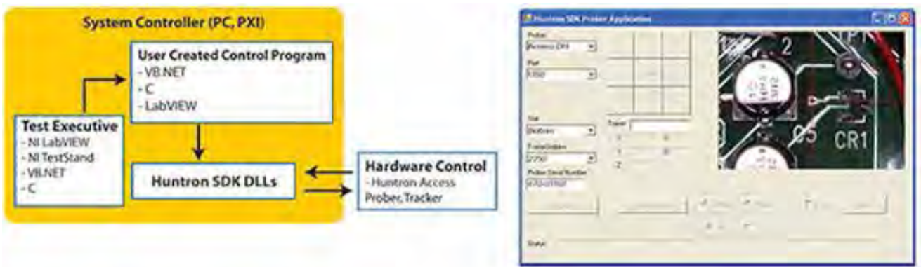
Hardware SDK Use block diagram and Sample Access Prober Camera application (image right) created using the Huntron Hardware SDK (click to enlarge image)
