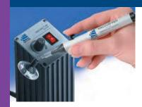
The SMD-VAC™ pick-and place tools provide a bench top vacuum generator. The whisper-quiet operation makes these the choice tools for many PCB assembly operations. Parts ranging in size from 0.0075" (0.19mm) up to 4" (102mm) can easily be handled.
