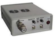
Pulse generators of FPG-P series have a rise time ranging from 100 ps to 1 nanosecond.
