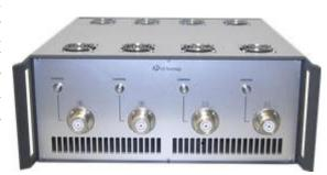
Output channels of FPG-X series pulsers can be synchronous
