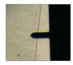
Video microscope used to locate surface features for scanning. The Vibrating Mode Cantilever is  $125~\mu$  long.
