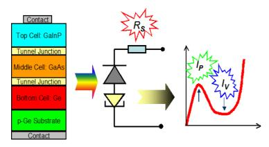
The RPV series test system is designed for the characterisation of concentrator tandem multi-junction solar cell. It is suitable for quick and accurate characterisation of the solar cell **internal Series Resistance, tunnel junction Peak and Valley current** non-destructively both in wafer and modules.
