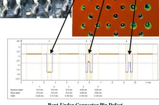
Bent-Under Connector Pin Defect (Precise measurement of each pin's depth within the PCB hole)
