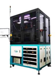
The VI500 is a high-speed, six-side vision inspection system for small parts, made of plastic or metal. Coming from a vibrator bowl input, parts are presented to the vision system on a specially treated glass carrier and sorted into bins.
